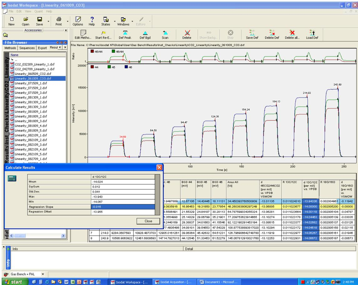
Figure 8: Carbonate Linearity Check (Using CO<sub>2</sub>)
